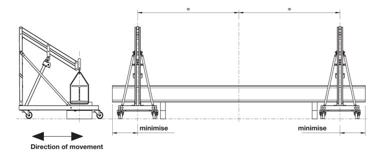
Once the heading fork and adapter, if required, are installed, the carrier (load) is to be lifted again **SYMMETRICAL** to the centre of gravity. Borings in the plates of the heading forks enable additional mounting of the carrier. It is recommended during the lift to always track the support to provide an additional safety device against tilting and falling. The lifting jacks must only be moved in their longitudinal direction with a lifted load!
