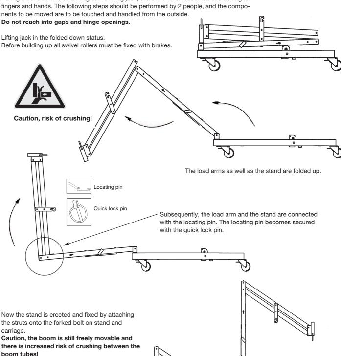
Subsequently the spindle is swivelled up and introduced to the slot accommodation of the lateral strap of the load arm. Now the heading fork can be
