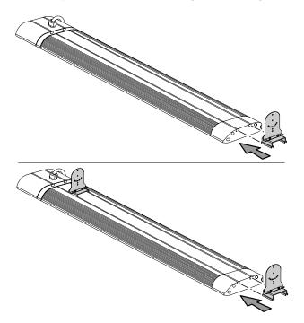
4. The brackets' position can be freely adjusted. The recommended distances are provided in the table below:
