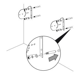
6. Check the mounting brackets for tight fit.
