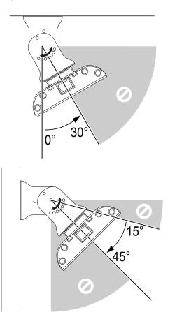
8. Connect the mounting brackets on the device to those on the wall / ceiling at the desired inclination angle. For each side, use two Phillips screws, two small hexagon nuts (M4) and spring washers (Ø 4.1 mm).
